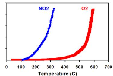
NO<sub>2</sub>-based systems are greatly favored because the (NO<sub>2</sub>) reaction takes place at lower temperatures (seen in most diesel engine exhaust), as compared to (O<sub>2</sub>) based systems needing higher temperatures for the reaction to occur.
